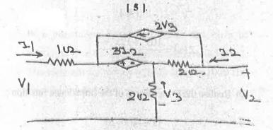
(c) Determine the ABCD (transmission) parameters for the network show below.
